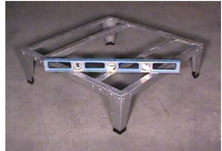
Make sure your stand is level. Thin pieces of metal, under the feet, may be used as shims.
