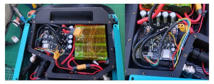
Here are some images of my bare bones build that only has a 4s2p booster and Tronic 250R. LED system and BMS were yet to be installed, however the wire harness had a 4pin JST Ready for balance wires from the boost pack and 3pin JST ready for the tail light input.
