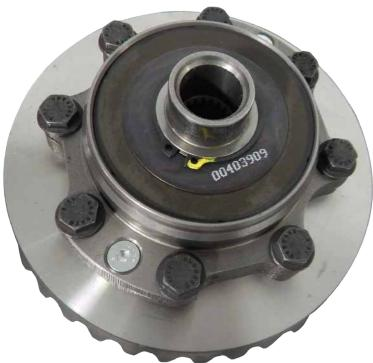
separate Clutch Pack from Ring Gear
