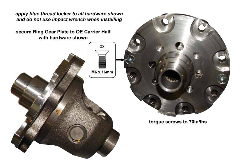
install Ring Gear Plate to Ring Gear with hardware shown
