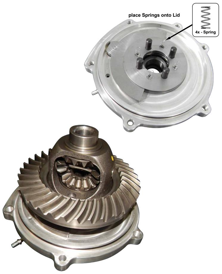
place Ring Gear Plate/OE Carrier Half assembly onto Lid
