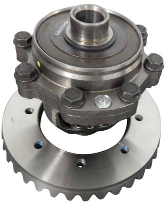
remove (2) countersunk screws from Clutch Pack
