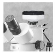
Thread the front of the camera onto threads of C-mount adapter.
