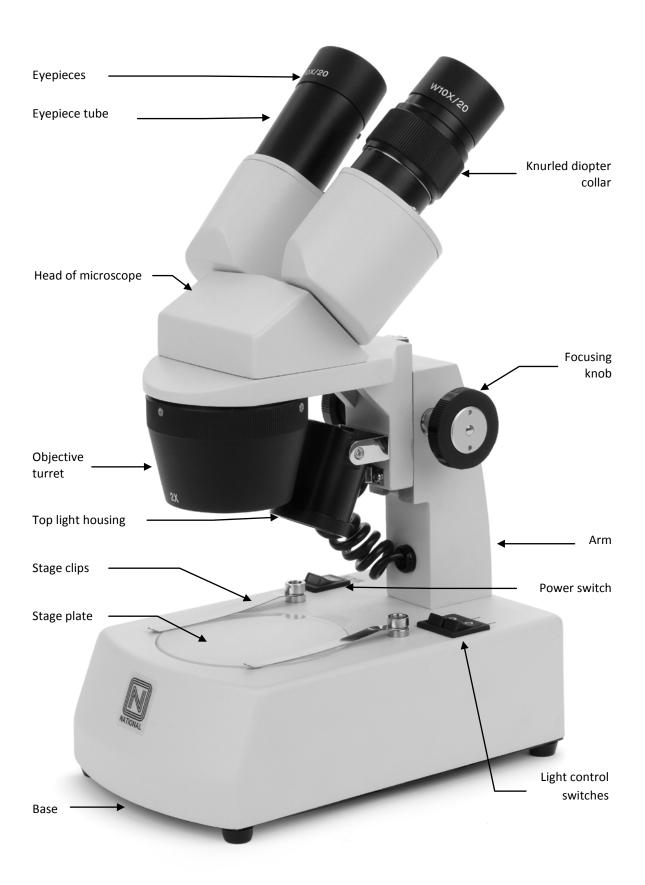
Stereoscopic microscopes are used for viewing 3-dimensional objects, inspection or assembly of small parts, and for dissection of biological specimen. They provide an upright, unreversed image which permits easy manipulation of the object being viewed while looking through the microscope. They are designed for viewing solid objects at low magnification, but they will also permit viewing of some transparent specimen slides.
