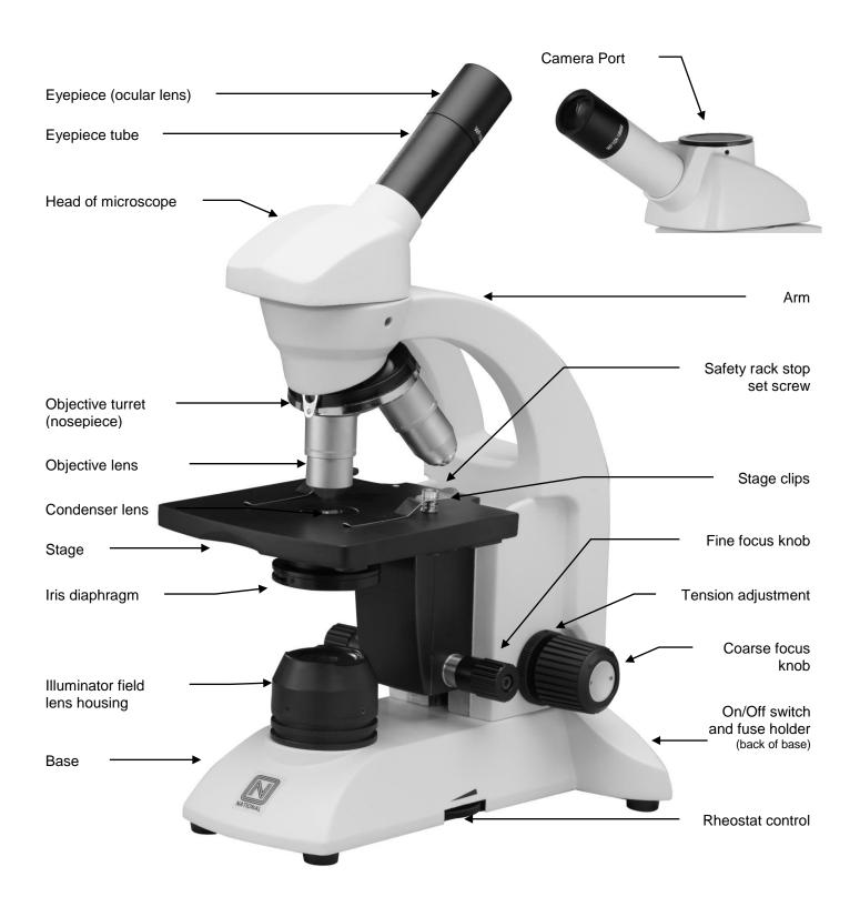
For optimum viewing satisfaction, follow these simple procedures. Nomenclature used to describe components and controls can be identified by referring to the diagram at left.
