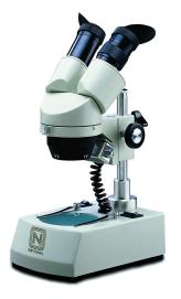
All the quality features and versatility of larger stereo microscopes, in a compact size that is more efficient for many uses. Choose low or high magnification simply by turning the objective turret. Viewing head is 45 degrees inclined and rotates 360 degrees so that user can position microscope conveniently in forward or reverse viewing position. Post mount permits head to be adjusted up or down to accommodate larger objects on stage.
