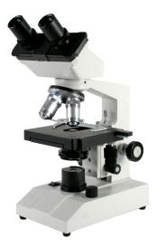
This popular choice for middle and high school instruction is enhanced with LED illumination. Delivers higher light efficiency than standard 20 watt tungsten bulb, and cool operating temperature prolongs specimen life when viewing live material. Precision optical and mechanical features combine with extra rugged construction and user-friendly features.
