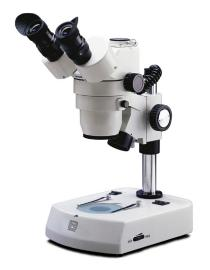
The convenience and versatility of viewing a large picture at 10x magnification, then zooming continuously all the way to close-up detail at 40x magnification. Upright, unreversed 3-dimensional image remains in focus throughout zoom range. Optional eyepieces and auxiliary objectives expand magnification range and working distances.
