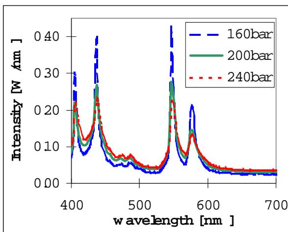
Figure 1: Measured UHP spectra of 1.3 mm lamps at 100 W depending on the mercury pressure.
