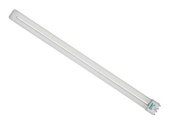
SYLVANIA DULUX L T5 lamps are high lumen, single-ended twin-tube lamps that provide lumen outputs similar to 2', 3' and 4' linear fluorescent lamps, yet are half the length. With lumen outputs up to 4800 and lamp efficacies up to 87 lumens per watt, these compact lamps can be used in indirect as well as direct applications.
