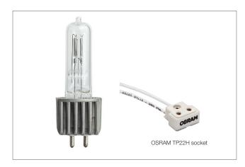
OSRAM HPL ULTRA PLUS (UCF) – An improved product line of the HPL family of lamps originally designed specifically for the Source Four® series of fixtures. The HPL ULTRA PLUS uses an ULTRA Compact Filament (UCF) design for maximum efficiency and life. The unique top bridgeless construction for lamps with ≤120 volts virtually eliminates filament shadowing, allowing for crisper images than ever before.
