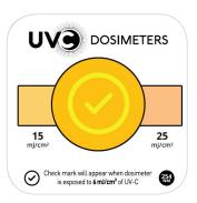
Designed for use with UV-C towers, upper air units, handheld devices, cabinets and more, the Quick Check UVC Dosimeter will reveal a check mark at 6 mJ/cm<sup>2</sup> and will continue to change color to indicate 15 and 25 mJ/cm<sup>2</sup>.
