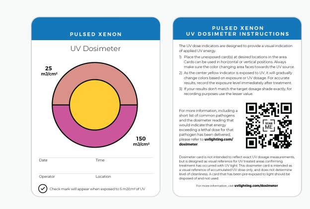
The pulsed-Xenon UV Dosimeter provides a visual indication of successful germicidal irradiation by revealing a check mark when exposed to 5mJ/cm<sup>2</sup> of broad-spectrum UV. Using a patented photochromic ink, the yellow center on the card changes color to indicate the intensity of the dose delivered from 25 to 150 mJ/cm<sup>2</sup>.
