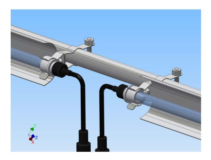
UVC lamps are provided with sure-seal moisture proof connectors on the power end of the lamp. Additionally, Lamp power cords can be provided in 8', 12', or 30' foot lengths for connecting each UVC lamp to the ballast control enclosure. Each lamp power cord has a mating sure seal connector to plug into the UVC lamp. Cord grips are provided with each lamp power cord for securing the power cord into the ballast control enclosure.
