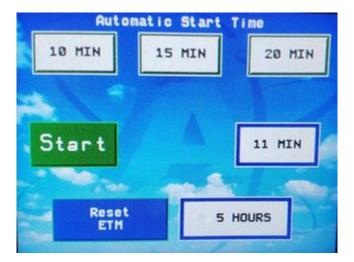
The three (3) time values across the top of the screen (10/15/20 minutes) are preprogrammed into the system. Select any one of these times and the Cycle Ready screen will be displayed.
