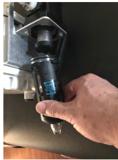
Push the black bulb up and give it a quarter turn to unlatch then pull down
