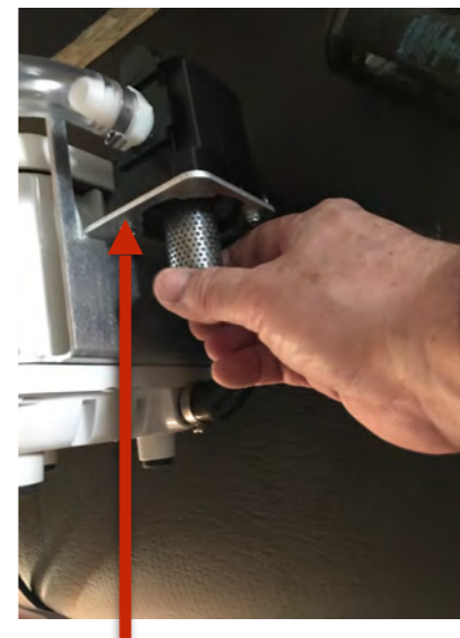
Unscrew the silver filter element. Screw on the new silver filter
