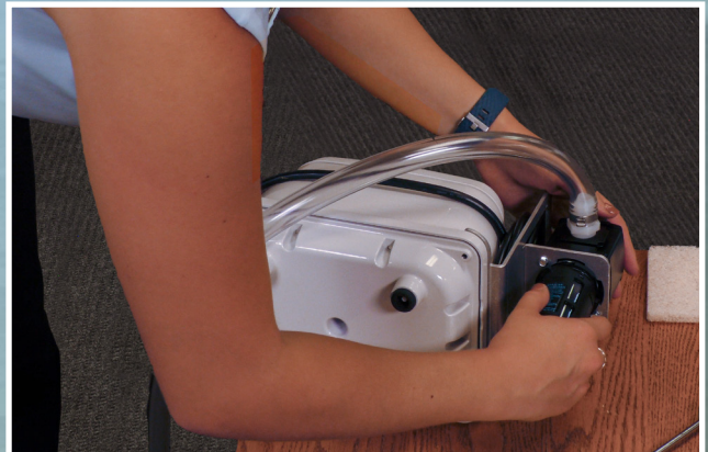
Put the black bulb back on pushing up and giving it a quarter turn to make sure it is securely connected.
