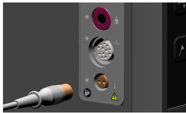
Figure 12 Connecting the Temperature Cable
