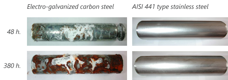
Example: Electro-galvanized carbon steel and AISI 441 type stainless steel after short and long salt spray test exposure.
