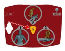
Fig. 4.8 Button to deliver the shock
