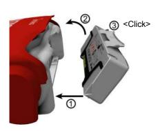
Fig. 3.1 Inserting the battery
