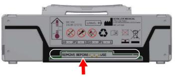
→ Remove the protective cap from the battery contacts before inserting the battery in the device.
