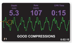
The AED 3 BLS can be easily configured to show the CPR Dashboard™ only (image to the left and top image above), or combined CPR Dashboard with ECG (middle and bottom images above). Red areas indicate the rate is too slow and/or depth too shallow in adult rescue mode.
