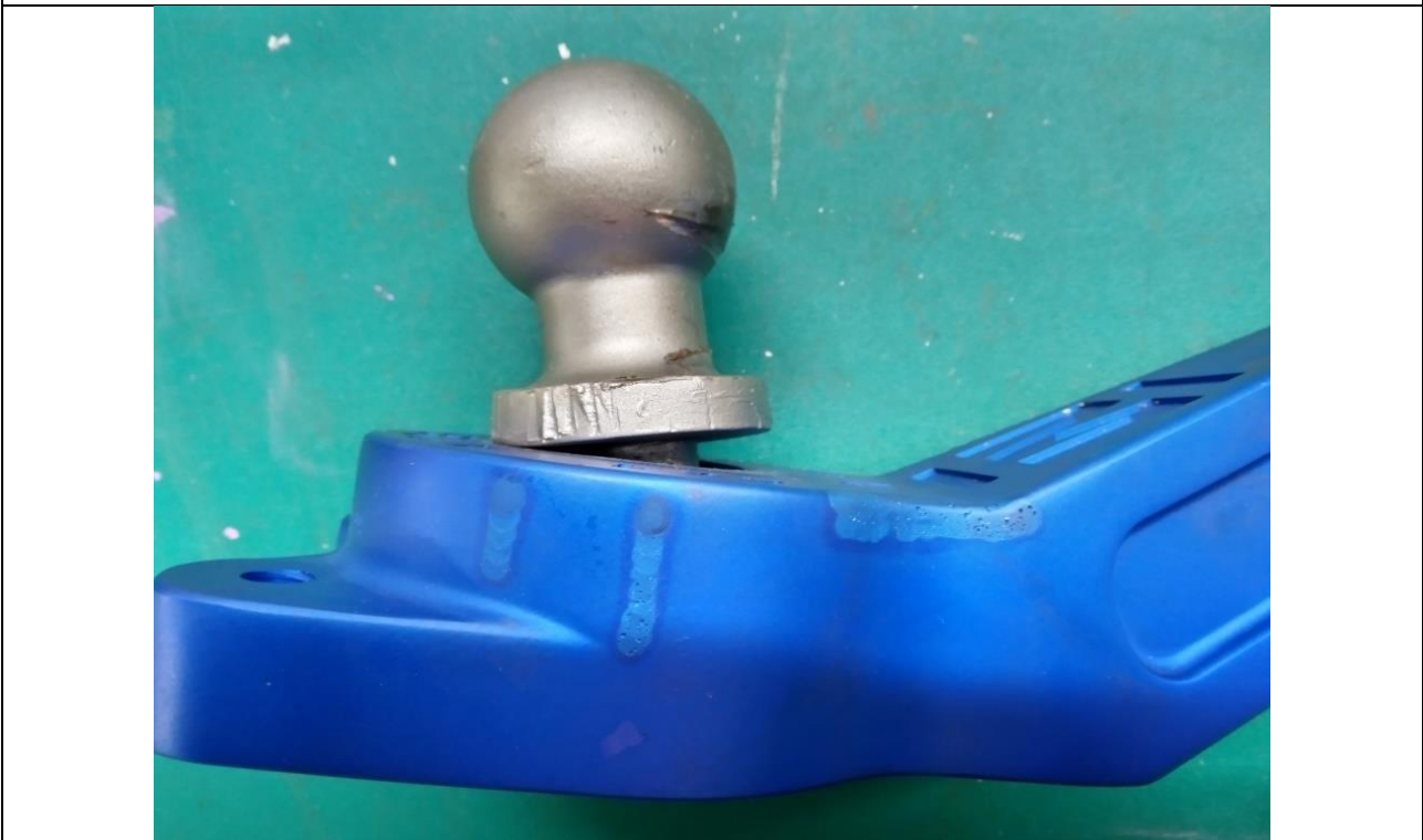
Figure 4: Photograph of the Trailer Hitch component after load test.
