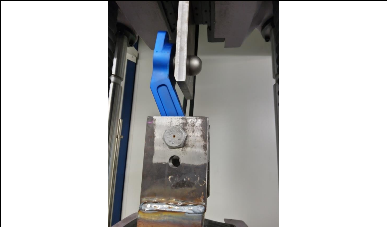
Figure 3: Photograph of the Trailer Hitch component during load test.
