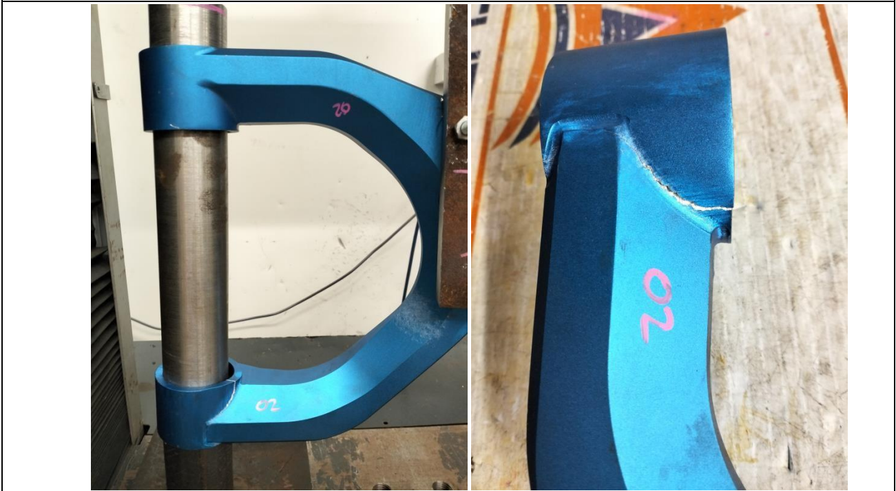
Figure 11: View of failure mode for sample 02.
