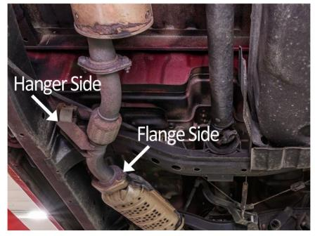
template hanger hole into your the exhaust hanger stud. Hold the template and check if template print and the catalytic converter flange line up for the two exhaust bolts.
