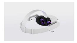
Detach the soft strap from the headset arms by placing your finger on the back of the strap's plastic casing, pulling it away from the headset with a slight twist downward. Unsnap both sides.
