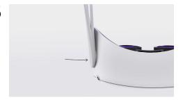
Snap on by gently applying pressure down the length of the strap.
