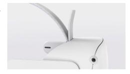
Unfasten the top strap and pull it though the bracket in the front of the headset.
