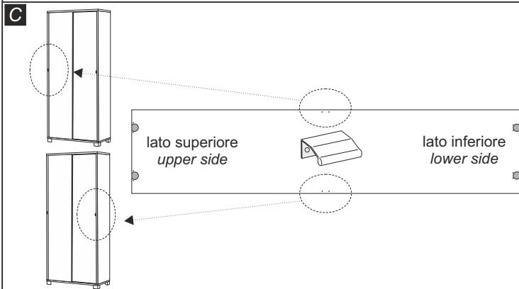
Fissare le maniglie (11) con le viti 4,5x16 (10) sulle ante (6) into the holes on the opposite side to the direction of opening.
