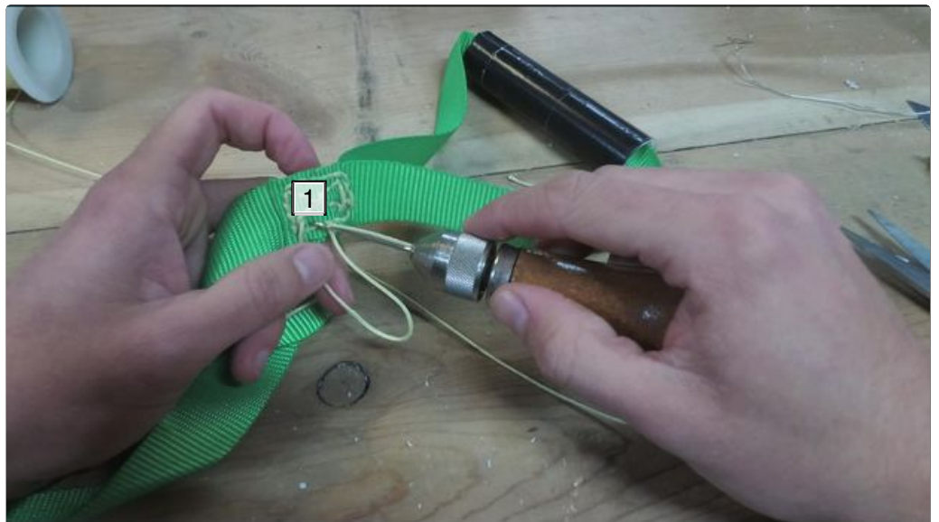
1. This is how the Box X stitch should look when it's done
