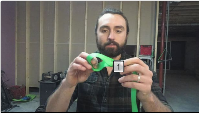
1. This is the loop on the end of the 4' strap, with heat shrink securing the sewn joint
