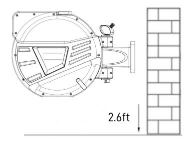
**Tips:** It is recommended to install the mounting seat 2.6ft from the mounting seat to the floor.
