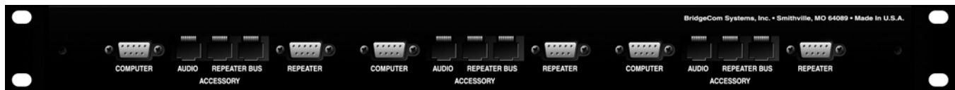
Rear View of three controllers in 1U chassis
