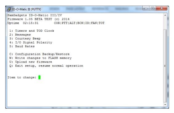
This is an example of what you will see in the main setup menu. Operation is as simple and intuitive as I could make it. To change a timer value or to set the clock, type 1 and hit the ENTER key. To add or change a message, type 2 and hit the Enter key, and so on.
