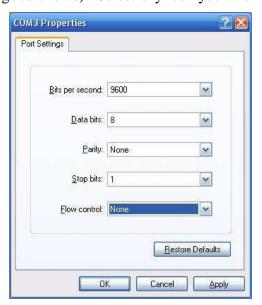
Modify the port settings for flow control = NONE. Since this is a USB connection, the bits per second setting does not matter.
