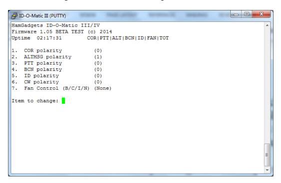
**COR and ALT MSG Polarity:** For each of the input signals (COR and ALT MSG), set the pin to 0 for active-LOW or 1 for active-HIGH. Active-LOW means the input signal is normally at a higher voltage level when idle, and goes to ground when active. Active-HIGH means it's normally grounded and goes to a positive voltage when active.
