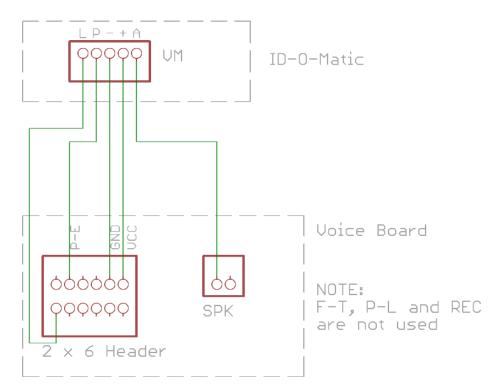
There are two speaker pads on the voice recorder board; you can use either one of them. The ID-O-Matic IV board has solder pads and holes for the five wires needed for the voice recorder board. The voice recorder board itself may have connectors installed. The connectors may be removed if you wish and wires soldered directly to the board, or you can wire up connectors to plug onto the board.
