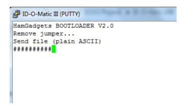
You'll see the LED blink rapidly alternating red and green, and there will be some hash marks printed as the file is loaded. It's best not to disconnect the board during this process, but you won't damage anything if you do. The bootloader will always be available, even after a failed
