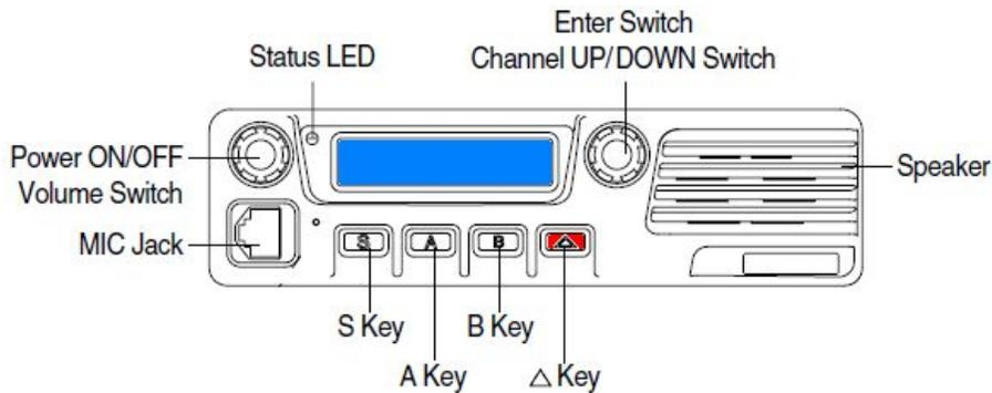
1. After power is applied, the radio is turned on by pressing and holding the volume control knob for approx 2 seconds. The radio defaults to VFO mode and the RX frequency is displayed. The volume control knob is located on the left side of the radio. Once turned on, the radio will cycle through displaying Model name, Firmware Version, and Channel name or Frequency depending on Mode. The associated icons will be displayed as well.
