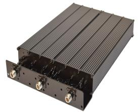
BridgeCom Systems BCD-220 utilizes six high-Q notch-type coaxial resonators with 2"-cross-section that results in small geometry advantages without compromising duplex isolation. Due to the right material choice and temperature compensated design, temperature stability is achieved. The resonators are made of extruded aluminum passivated inside and outside with the galvanized steel chassis and PTFE insulation has been applied in the coaxial cables and in the connectors.
