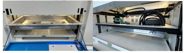
(Optional) The ability to secure your twister tray with supplied ¼" carriage bolts and wing nuts. Insert provided carriage bolts in the holes in front of the tray and secure to the honeycomb frame with supplied washers and wingnuts, **do not over tighten**! This eliminates any movement of the tray when engraving. This provides confidence that you won't move the tray when changing tumblers.
