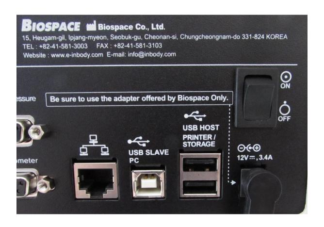
4. Once the USB thumb drive has been inserted and press the top left corner consecutively until you hear a chime. (NOTE: Please unplug the printer from the InBody before pressing the top left corner) .This indicates that the data is being copied. Shortly after, you will hear another chime indicating that the transfer has been complete.
