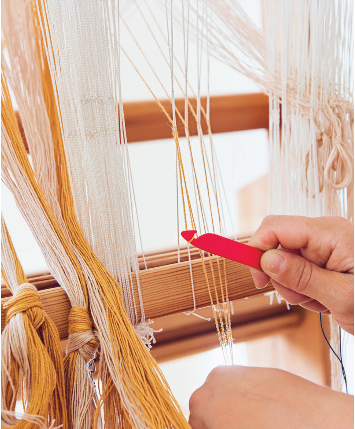
Threading with a threading hook. The ends that have been threaded are to the right of my hand, and those waiting to be threaded are to the left.
