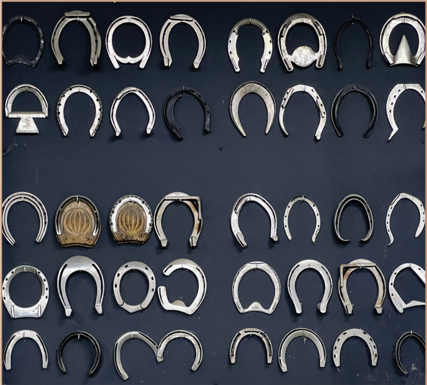
3.1 C Hand-forged shoes like these by Henry Asmus show how farriers can customize horseshoes to treat a myriad of hoof problems. These were specifically for driving horses.
