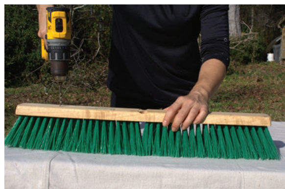
9.73 Preparing a DIY scratching post by pre-drilling holes in the brush for easier attachment to the post.
