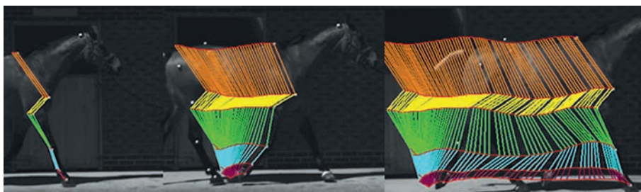
Photo 7.4 The computer software tracks the markers as the horse moves, to obtain a visual representation of how the limb moves throughout one stride. (Courtesy of www. quintic.com)
