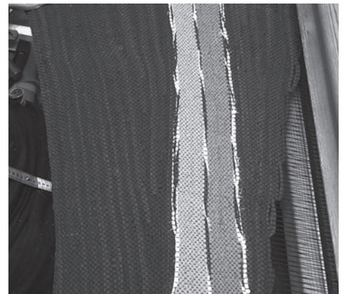
9. The second angled half on the other side of the stripe is woven like the first half. Pull the rug forward so it lines up with the breast bar and continue with the next vertical straight section, see picture 2.
