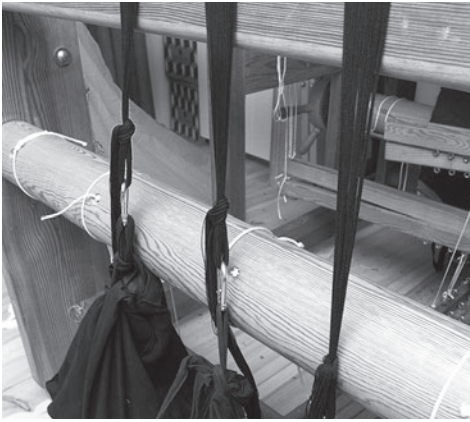
1. Divide the warp and suspend weights of ca 1.5 kg each from each section.
