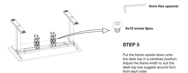
Once in position, tighten the M6x10 screws to set the frame width
