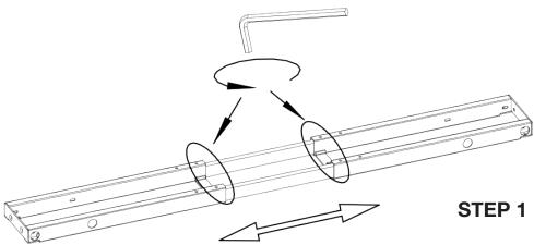
Loosen the 4 screws using the hex spanner, so the frame can adjust to the desk top size as/when needed.
