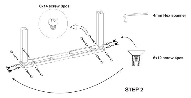
Attach legs to the support beams using the parts shown
