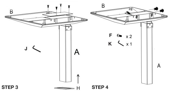
Assemble the bottom cover (Refer to Step 1)
