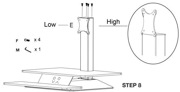
Part E (VESA monitor mount) can be assembled facing up or down for increased height range.
