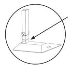
Insert Part H in place around the main column where it meets the base (Part B). Use 2 x screws (Part F) on each to secure Part A main column at the rear. Then fully tighten all 6 screw positions (including the first 4 screws from Step 2).
