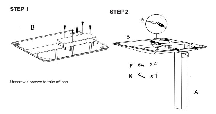
Insert main column (Part A) through Part B (base)
