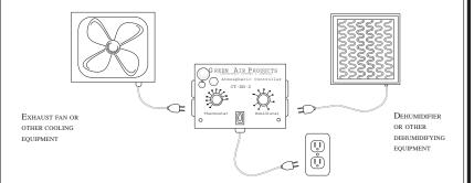
This example shows the basic independent function of the CT-DH-2 for the purpose of operating equipment intended to cool and dehumidify.
