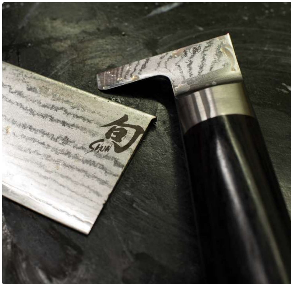
Above: A Shun Classic Chef's blade is cut for a cross-section.
