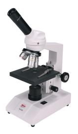
The M2250 Series is ideal for a wide variety of educational applications and built to withstand student use. This series has locked-on stage clips, eyepiece, objectives (sealed 40X), and a slip-clutch focusing system to protect gears from over-focusing. The M2250 Series is offered with cool and efficient LED illumination. This model can be used corded or cordless.
