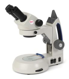
The SM100 Series features energy-efficient variable LED illumination with six light setting combinations, one-touch spring loaded stage clips, and right eyepiece diopter focusing adjustment. These models can be used corded or cordless. Ideal for high school classrooms and up.
