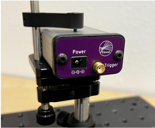
Figure 2. Back panel showing SMA pulse trigger and barrel power connector.
