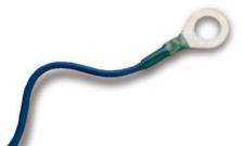
Keep the heat source or product moving. Do not concentrate the heat in one spot. Keep the heat source at least one inch away from tubing. Use a low-intensity heat source such as a hot air gun, oven, infrared heat source, or soft (yellow) flame.
