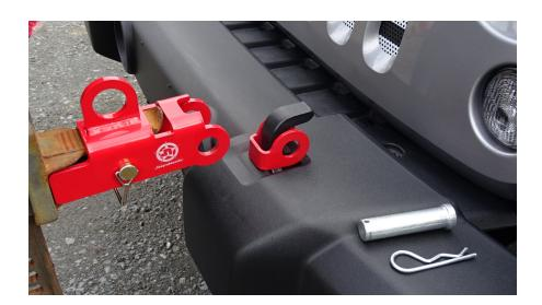
3). Slide the SAM-U adaptor over the locking retainer key, insert the clevis pin through the SAM-U and the locking retainer key, and secure the clevis pin in place with the wire clip. Making sure the jack is on a vertical position, your ready to jack the vehicle up.
