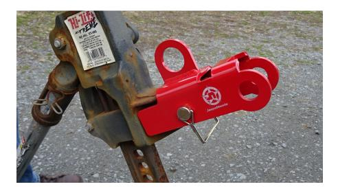
2). Place the locking retainer key, flat side down onto the factory recovery hook as as shown on the photo below
