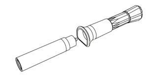
2. Attach the cream cylinder to the main device. Press down until you hear a click
