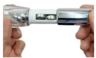
3. Replace the battery. Check the polarity markings (+)(-) and insert the new battery correctly.
