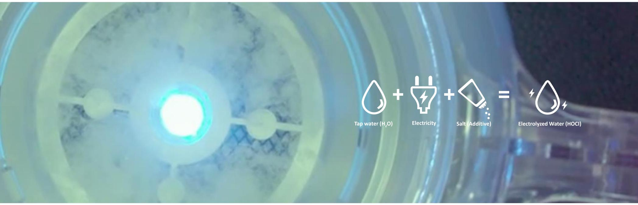
The special technology in Homeguard enables tap water to become sterilizing and deodorizing solutions by electrolysis. This is called electrolyzed water. The electrolysis of tap water (Cl<sup>-</sup> + H<sub>2</sub>O  $\rightarrow$  OCl<sup>-</sup> + 2H <sup>+</sup> 2e<sup>-</sup>) which contains a small amount of chlorinated ion (Cl<sup>-</sup>) will generate hypochlorous acid.
