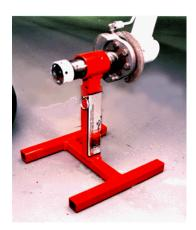
11. **TO LOWER:** Slowly turn the RELEASE VALVE counter clockwise with the jack handle and slowly lower the jack. When the tire is resting on the ground and the axle is free of the jack, remove the jack,
